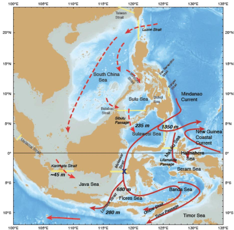
Figure 1. Flow pattern of components of the Indonesian Throughflow. Sill depths are given for the major choke points and the main passages and seas are indicated.
